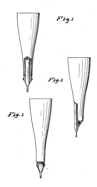
Fig. 1 is a front elevation on enlarged scale of a nib section for a fountain pen showing my new design.
