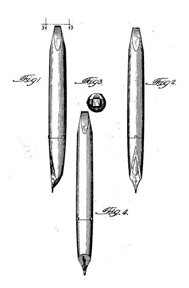
Figure 1 is a side elevational view of a fountain pen or similar article showing our new design;
